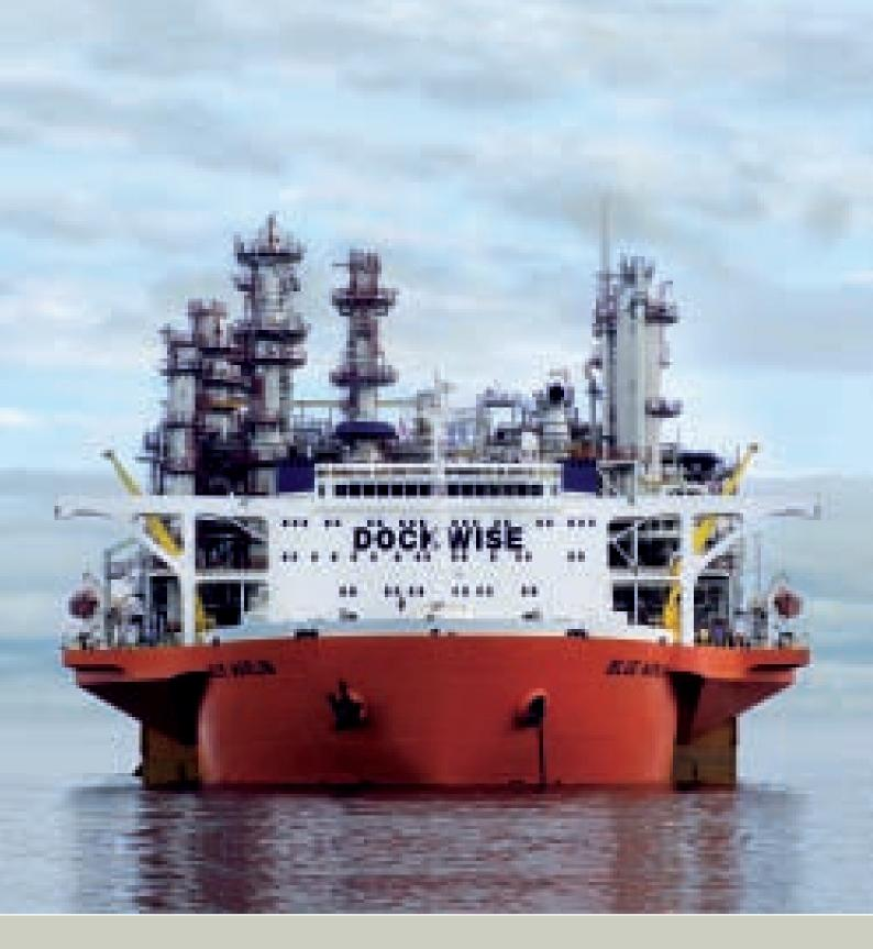
Natural gas plant transported by ship to Norway // It weighs 35,000 tonnes and is bigger than a football field. The centerpiece of the largest natural gas liquefaction plant in Europe on its way from Cadiz in Spain to its destination, Hammerfest in Norway. On the biggest bulk cargo ship in the world, the Blue Marlin, the plant covered around 2,700 nautical miles in ten days.
