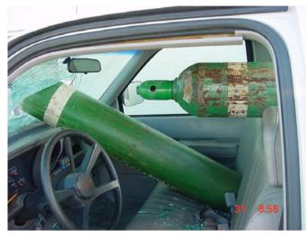
Some gases such as Propane, Carbon dioxide (CO<sub>2</sub>) and Acetylene should not be transported lying down as the gas in these cylinders is in liquefied form, or as in the case of Acetylene dissolved in acetone. Consequently, there is a very real risk of an escape from the valve threads and gas then collecting in sufficient quantities to form an explosive or asphyxiant mixture inside the vehicle
